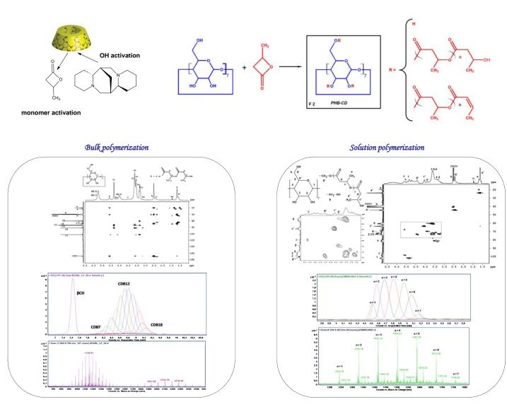
• Average length of the PHB chains ~ 3 monomer units by NMR and 12 by LC ESI MS • Cyclodextrins substituted with ~ 4 PHB chains having in average 3 monomer units
