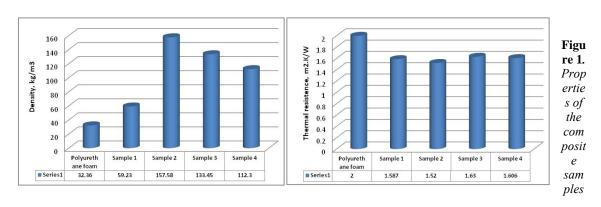
The analysis of the obtained composite samples showed multilayer structures of polyurethane foam, mineral wool and cellular polyethylene (samples 3 and 4), with properties of sound insulation, thermal insulation and high flexibility. In order to reduce the degree of flexibility, internal metal structure of the aluminum sheet has been introduced into the foam layer.
