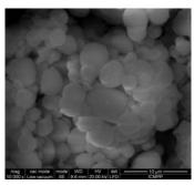
Fig. 1. SEM image of VCL-MAc microparticles
