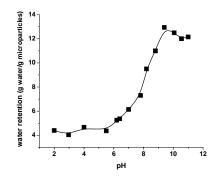
Fig 2. Influence of the pH on the swelling characteristics of VCL-MAC microparticles in water
