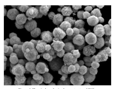
Figure.1 Chemical synthesized nanostructured WO<sub>3</sub>.
