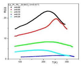
Variation of the resistance vs temperature and Pb concentration. The samples were cooled and measured in a magnetic field of 4300 Oe.
