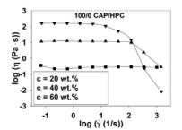
Figure 1. Log-log plots between dynamic viscosity and shear rate for CAP/HPC blends at different concentrations in N,N-dimethylacetamide.
