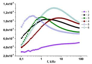
Figure 1. Frequency dependences of M" for the unmodified CPU-0 (1) and CPU-KNT, modified with 1% wt\_of Cu(acac)<sub>2</sub> (2), Co(acac)<sub>3</sub> (3), Cr(acac)<sub>3</sub> (4),  $[Cu_3Mn(L)_4(CH_3OH)(H_2O)_3]Br \cdot 3H_2O$  (5) and  $[Cu_3Mn(L)_4(CH_3OH)_3]I_3$  (6), where L is the product of condensation of salicyl aldehyde with ethanolamine.
