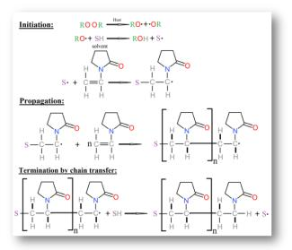
Figure 2. Polymerization of VP in organic solution.
