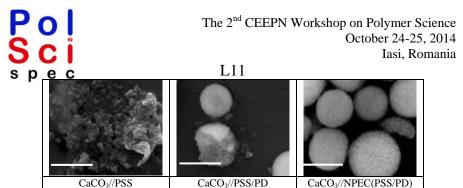
Figure 2. SEM images of some samples after EDTA treatment; PSS – poly(sodium styrene sulfonate), PD –poly(dimethyldiallylammonium choloride). Scale bar – 5  $\mu$ m.
