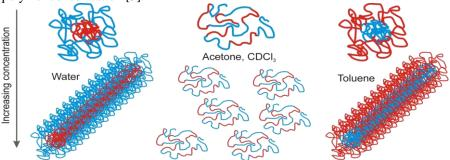
Figure 4. AIPs self-assembly by increasing concentration in aqueous and organic solutions.
