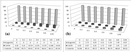
Figure 2. Polymorph content of CaCO<sub>3</sub> based microparticles template by (a) *in-situ* mixing of complementary polyelectrolytes or (b) preformed NPECs as a function of  $n^+/n^-$ .
