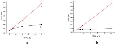
Figure 2. Density versus TEOC content dependence for PI composites of series 1 (a) and series 2 (b). Additive (1) and experimental (2).
