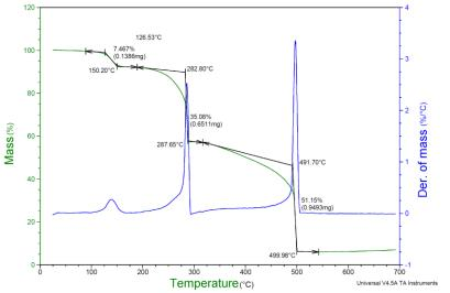
Figure 2. Thermogravimetic analysis and thermo differential analysis data of the polymer microspheres Expancel 461WE 80 d36.
