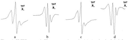
Figure 1. SP EPR spectra in PI nanocomposites series 1 (a,c) and series 2 (b,d) for initial PI (a, b) and containing 50% wt of TEOS (c,d).
