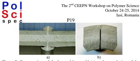
Figure 3. Cross sections of the hot tool butt weld (a), and general view of the destroyed specimen after tensile test (b).
