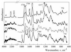
Figure 1. FTIR-spectra of individual PAI (1), porous PAI/PU film(2), non-porous (precursor) PAI/PU= (70/30) wt.% film (3) and individual PU (4).
