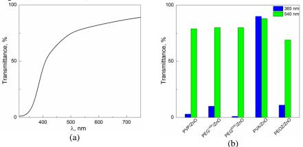
Figure 2. Optical properties of nanohybrid obtained: (a) UV-vis spectrum of PVP/ZnO and (b) transmittance values of polymer/ZnO nanohybrid at fixed wavelength.
