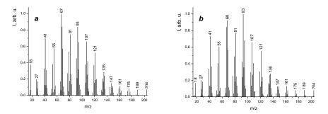
Figure 1. Mass-spectra of volatile products of thermal destruction of liquid rubbers obtained with HP as an initiator: a - in isopropanol; b - in n-butanol.
