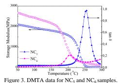
that this curing schedule allows effective reinforcement of CER network by MMT nanofiller. The considerable decrease of  $T_g$  and height of tan  $\delta$  values is observed as well and post-curing starts at  $T > 250^{\circ}$ C (Fig. 3).
