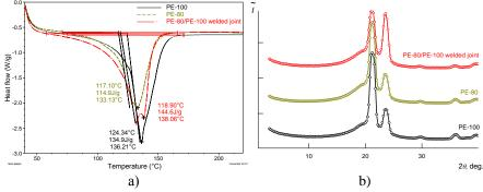
Figure 3. DSC (a) and WAXS (b) spectrums of pure PE-80, PE-100, and of their weld PE-80/PE-100.
