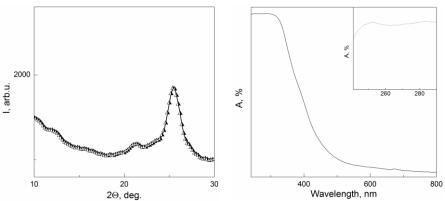
Figure 1. XRD pattern (a) and UV-DRS curve of catalyst with  $TiO_2$  content of 50 % (by weight).
