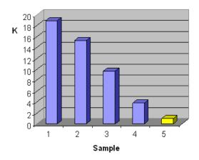
Figure 1. The relative hydroabrasive wear of stainless steel and polymers MM 2000 (1), MM 2800 (2), MM 3550 (3), MM 4400 (4), steel 12X18H10T (5), **K** - coefficient of relative hydroabrasive wear
