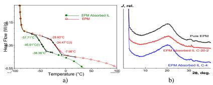
Figure 5. Calorimetric (a) and WAXS (b) spectra of pure and doped EPM.
