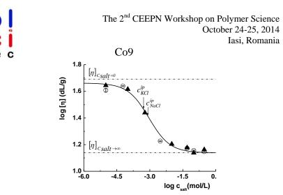
Figure 1. Dependence of the intrinsic viscosity as a function of the salt concentration for xanthan aqueous solutions at  $25^{\circ}$ C; full triangle – NaCl; open circle – KCl [6].
