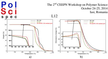
Figure 2. Thermogravimetric (a) and thermomechanical (b) results of pure PE-80, PE-100 and their PE-80/PE-100 weld.
