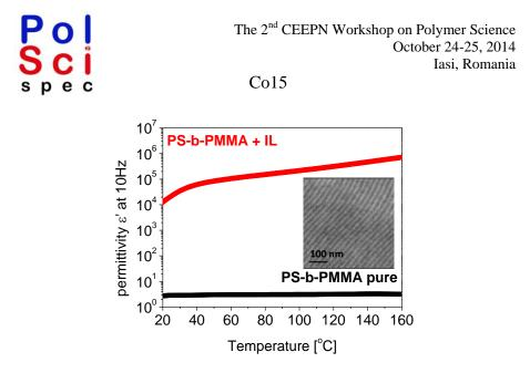
Figure 1. The permittivity value of pure PS-b-PMMA and of PS-b-PMMA doped with an ionic liquid. Insertion: sequence of insulating and conductive polymer nano-layers.
