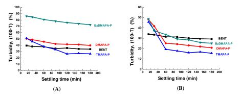
Figure 1. Turbidity data for BENT alone, BENT with DMAPA-P, BENT with TMAPA-P and BENT with BzDMAPA-P in aqueous solutions without (A) and with 0.5M NaCl (B).
