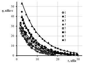
Figure 1. Relation of dynamic viscosity  $\eta$  to shear stress  $\tau$  of composites containing 4,3 % of the following plasticizers: DOP (1, 2), NDA-ET (3, 4), PA-ET (5, 6), HSO-ET (7, 8) at temperatures of 40 °C (1, 3, 5, 7) and 50 °C (2, 4, 6, 8)
