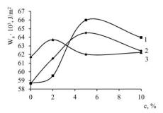
Figure 1. Effect of polymer-modifier content on the adhesion between PVCplasticizer: 1,2 - dibutyl phthalate (DBP); 3 - di-2-ethylhexyl phthalate (DEHP); 1,3 - PS; 2 - ABS
