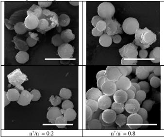
Figure 3. SEM images of some CaCO<sub>3</sub>/polymers microparticles after EDTA treatment: top line - CaCO<sub>3</sub>//PVS/PD, bottom line - CaCO<sub>3</sub>//NPEC(PVS/PD); scale bare 10  $\mu$ m.
