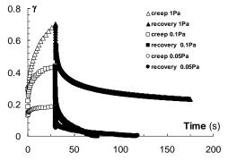
Figure 1. Creep-recovery tests for 0.4 g/dL xanthan aqueous solution at 37°C.
