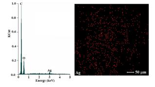
Figure 1. The EDX pattern, quantification data and corresponding EDX map collected from F1+2.5% Ag film.
