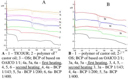
Figure 1. Temperature dependences of heat capacity castor oil- styrene BCP. Beginning a curve 2, all the subsequent ones are displaced relative to the ordinate axe 1.1.
