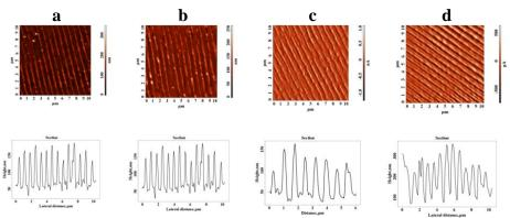
Figure 1. AFM images of the structured surfaces and diagram profiles of an azopolyimide film after laser irradiation with 10 mJ/cm<sup>2</sup> and 45 mJ/cm<sup>2</sup>, by using 10 and 100 pulses.
