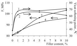
Figure 3. Effect of filler content of polymer-silicate composite on surface hardness and Vicat softening point. 1, 3 - polymersilicate composite modified by polyvinylpyrrolidone; 2,4 polymer-silicate composite.
