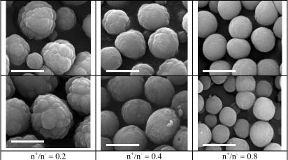
Figure 1. SEM images of  $CaCO_3$  based microparticles template by complementary polyelectrolytes as a function of molar ratio between ionic charges: top line -  $CaCO_3//PVS/PD$ , bottom line -  $CaCO_3//PVS/PD$ ; scale bare 5 µm.
