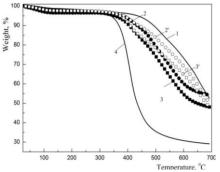
Figure 2. TGA curves obtained for nonporous PAI/PU films with PU content, wt.%: 0 (1), 10 (2), 20 (3) and 100 (4) (2' and 3' corresponding additive curves.).
