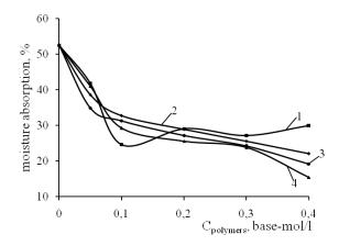
Figure 2. The influence of polymer concentration and the way of his addition (1, 4 - into the liquid glass 2, 3 - into the solution CuCl<sub>2</sub>) on the moisture absorption of polymer-silicate materials; 1, 2 - PVP; 3, 4 – PVA.
