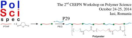
Figure 2. Scheme and reaction of the AIPE-2 synthesis.
