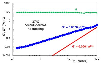
Figure 2. The viscoelastic parameters as a function of oscillation frequency for a solution with 15% polymer and composition of 50PVP/50PVA (37 °C, 1Pa).
