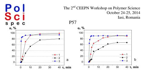
Figure 1. Kinetic curves of 1 - cycloaliphatic epoxy groups conversion, 2 - aliphatic epoxy groups conversion, and 3 - double bonds conversion under the sunlight (*a*) and under the UV lamp (*b*) in a system Epoxide 1 - TEGDM.
