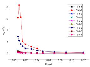
Figure 1. The concentration dependence of viscosity of polyionens based on tetrahydro-1,4-oxazyn and epoxide derivatives of 1,2-epoxy-4.7-dioksononen-8 in aqueous solutions: 1 – PI-1-1, 2 – PI-1-2, 3 – PI-1-3, 4 – PI-1-4, 5 – PI-2-2, 6 – PI-2-3, 7 – PI-3-3, 8 – PI-4-3, 9 – PI-4-4.
