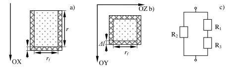
Figure 1. a) – averaged element; b) – cross-cut of averaged element in YOZ plane; c) – equivalent scheme of averaged element heat resistances.
