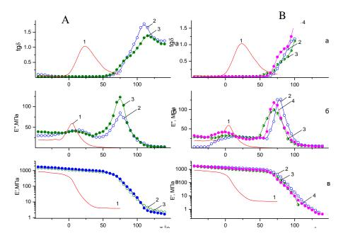
A - 1 – polymer of castor oil; BCP of based on OAICO 2/1: 2 - BCP 1/143; 3 -BCP 1/400.
