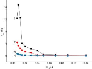
Figure 2. The concentration dependence of viscosity of PI 1-2 at different temperatures: 1 - 25 °C, 2 - 35 °C, 3 - 45 °C, 4 - 50 °C.
