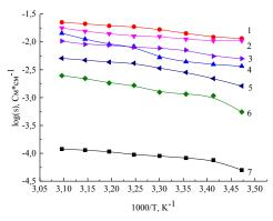
Figure. Temperature (1000/T) dependence of ionic conductivity (logσ) ILPQSAM: 1–C-1-7, 2–C-8-1, 3–C-1-3, 4–C-1-9, 5–C-1-2, 6–C-1-1, 7–C-1-8
