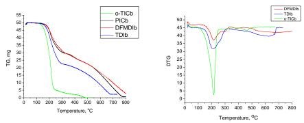
Figure 2. Thermogravimetric analysis of  $\varepsilon$ -CL blocked adducts.
