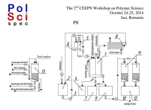
Figure 1. Process flow diagram for methyl FAEs production and catalyst regeneration unit:
