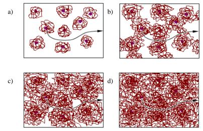
Figure 2. Morphological model of the creating process of the polymer structure of the epoxy resin hardened by heteropolyacid due to the homopolymerization mechanism. The arrows show proton movement under voltage to the negative charged electrode.
