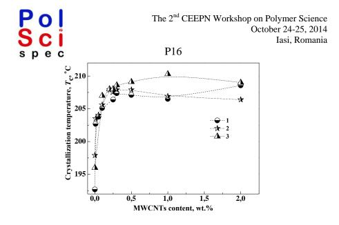
Figure 1. Effect of MWCNTs content and molding technique used on crystallization temperature  $T_c$  of the PBT crystallites in the PBT/MWCNTs nanocomposites studied: 1 – extrusion strand (series 1); 2 – hot pressing (series 2); 3 – injection molding (series 3).
