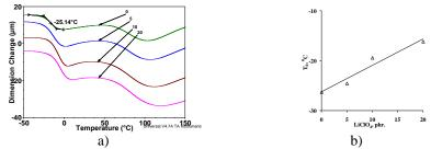
Figure 1. TMA curves (a) and dependence of the glass transition temperature of the epoxy system based on DEG obtained on contents of  $LiClO_4$  (b).
