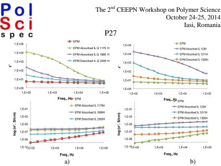
Figure 4. Sorption/desorption processes of IL Q (a) and IL 2Q (b) in EPM by electrical and dielectric studies.
