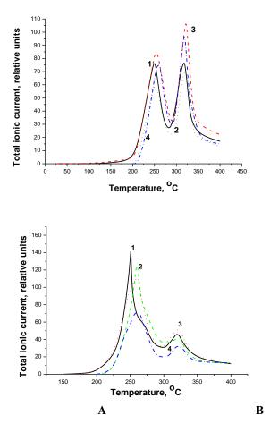
Figure 1. Thermograms on total ion current of releasing volatile products of thermal destruction of EG-80A (A) and TT-1085A (B) before (1) and after incubation with *Ps. denitrificans* (2); *Ps. fluorescens* (3) and *Y. lipolytica* (4).
