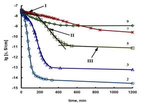
Figure 1. Kinetics of the hardening process of the EPTP systems studied by electrometric method. Numbers near curves show water content in the reactive mixture.
