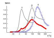
Figure 1. The temperature dependences of mechanical loss tanó for PU (1), PHEMA (2), IPN-1 (3), and IPN-2 (4).
