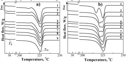
Figure 2. DSC thermograms for PBT/MWCNTs nanocomposites (extruded strands) with different content of MWCNTs, wt. %: 1 - 0; 2 - 0.01; 3 - 0.05; 4 - 0.1; 5 - 0.25; 6 - 0.3; 7 - 0.5; 8 - 1.0; 9 - 2.0; a)  $1^{st}$  heating scan; b)  $2^{nd}$  heating scan.
