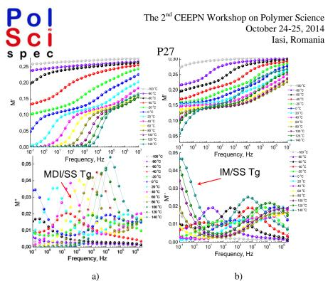
Figure 3. Dielectric modulus spectra of lowly (a) and highly (b) cross-linked EPM.
