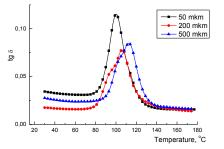
Figure 2. Temperature dependence of the tg  $\delta$  for steel adhesive joint.
