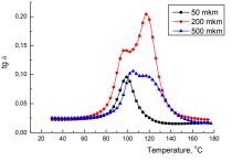
Figure 3. Temperature dependence of the tg  $\delta$  for copper adhesive joint.
