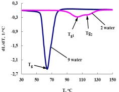
Figure 3. Differential TMA curves of polymers hardened by PTA with 2 and 9 weight parts of water in the reactive mixture.
