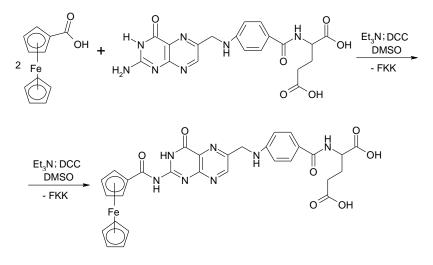
FFC was obtained as a brown powder with  $t_m 449 - 455$  K, with practical yield 67.2 %. The chemical structure of the reaction products confirmed by inftared method and 1H NMR-spectroscopy.
