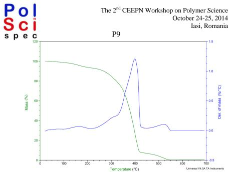
Figure 1. Thermogravimetic analysis and thermo differential analysis data of the polymer matrix based on the mixture of acryl-urethane water dispersions.
