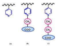
Figure 1. Structural units of poly(4-vinylpyridine) (a), P4VPB-1 (b) and P4VPB-2 (c).
