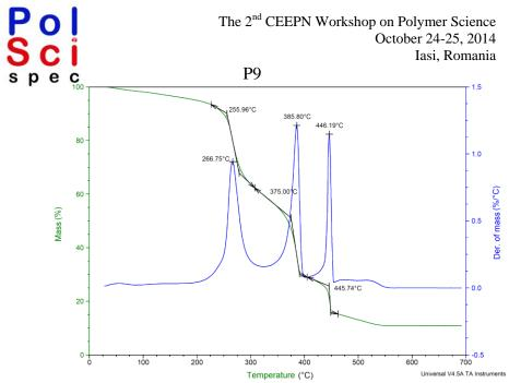
Figure 3. Thermogravimetic analysis and thermo differential analysis data of the thermal protection material with containing of microspheres 19% and density, 0.6  $g/cm^3$ .
