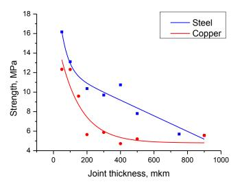
Figure 1. Influence of the joint thickness on overall strength for different substrates.
