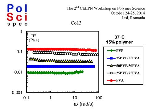
Figure 1. Complex viscosity obtained in frequency sweep experiments at 37 °C for 15% polymer solutions with different PVA/PVP compositions.
