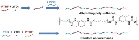
Figure 3. Scheme and reaction of the AIPU synthesis.
