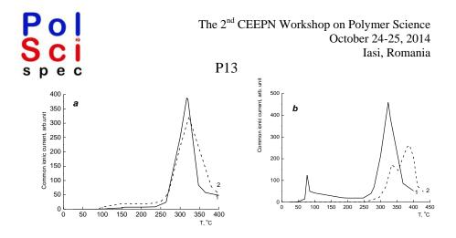
Figure 2. The temperature dependence of common ionic current of volatile product emission at thermal destruction of liquid rubbers, obtained with various initiators: a) 1 - AIBN; 2 - HP in isopropanol; b) 1 - HP in n-butanol; 2 - ACP.
