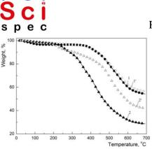
Figure 3. TGA curves obtained for precursors PAI/PU containing 10 (1) and 30 (2) wt.% of PU and corresponding porous films (1') and (2'), respectively.
