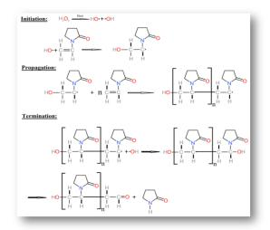
Figure 1. Polymerization of VP in aqueous solution.
