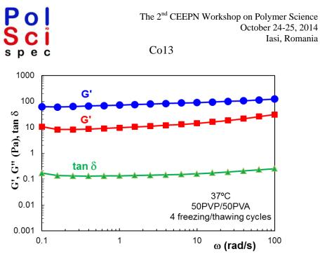
Figure 3. The viscoelastic parameters as a function of oscillation frequency for the same system as in Figure 2 after 4 freezing/thawing cycles (37 °C, 1Pa).
