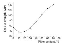
Figure 1. Tensile strength of composite based on modified used PET matrix and reinforced by glass fibers depending on glass fiber content..
