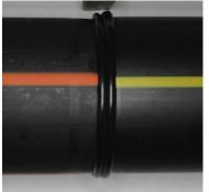
Figure. 1. Dissimilar pipes weld (PE80 and PE-100, 63 mm diameter).
