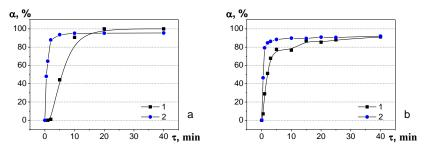
Figure 2. Kinetic curves of 1 - aliphatic epoxy groups conversion, 2 - double bonds conversion under the sunlight (*a*) and under the UV lamp (*b*) in a system Epoxide <math>2 - TEGDM.
