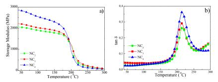
Figure 2. DMTA data for NC<sub>2</sub>, NC<sub>3</sub> and NC<sub>4</sub> samples.
