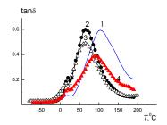
Figure 2. The temperature dependences of mechanical loss tan $\delta$  for OII-1 (1), OII-2 (2), OII\_3 (3), and OII\_4 (4).
