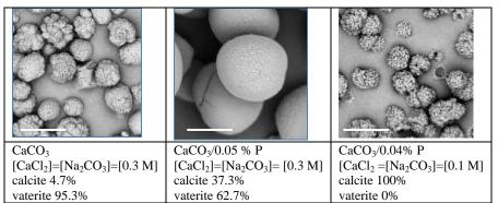
Figure 1. SEM images for some CaCO<sub>3</sub>/polymer samples; P = poly(2-acrylamido-2-methylpropanesulfonic acid - co - acrylic acid); scale bar - 10 µm.
