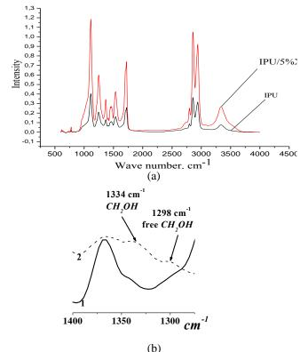
Figure 1. IR-spectra: IPU and IPU/5%Xn - (a); IPU/5%Xn (1) and Xn (2) – (b)
