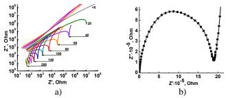
Figure 3. Z"/Z' plots of the epoxy system with 5 phr LiClO<sub>4</sub> at temperature range from -60 to +200 °C in double logarithmic coordinates (a) and in the coordinates Cola-Cola at temperature 30 °C (b).
