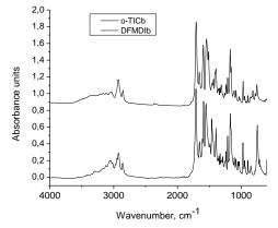
Figure 1. FTIR spectra of  $\varepsilon$ -caprolactam blocked o-tolyl isocyanate and  $\varepsilon$ -caprolactam blocked diphenylmethyl diisocyanate..
