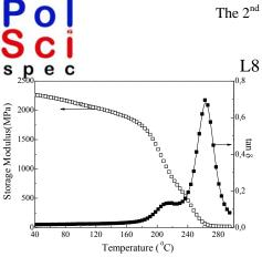
Figure 1. Storage modulus (*E'*) and tan  $\delta$  versus temperature for NC<sub>1</sub> sample (at frequency 10 Hz).
