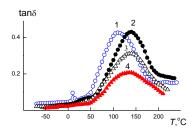
Figure 3. The temperature dependences of mechanical loss tan $\delta$  for OII-5 (1), OII-6 (2), OII-7 (3), and OII-8 (4).
