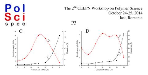
C The dependence of mechanical properties of system (DER 331 + CC DEG-1) + DETA (schedule I):1 - tensile strength, 2 - elongation
