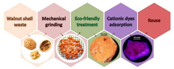
**Figure 1.** Schematically representation of walnut shell processing for the adsorption of Crystal Violet from aqueous medium.
