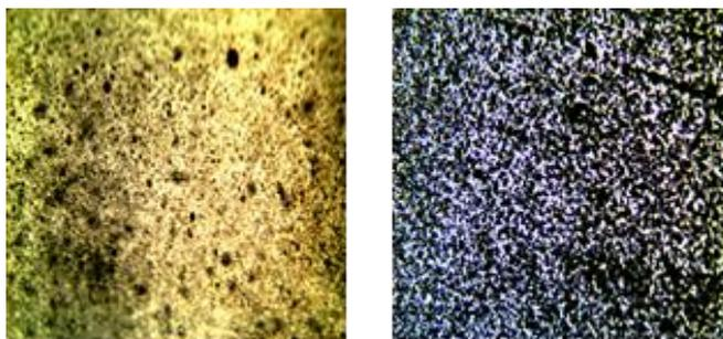
**Figure 2.** Profiler of the roughness measurements profiles for neat (left), and treated in air plasma polyurethane samples (right)
