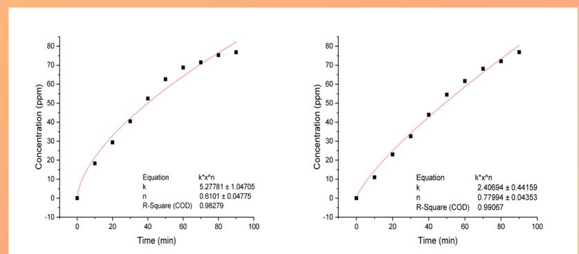
Figure 4. The release of piroxicam from Xa-Alg and XaAO-Alg.
