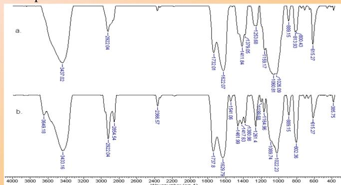
Figure 1. FTIR spectra for Xa (a) and XaAO (b).
