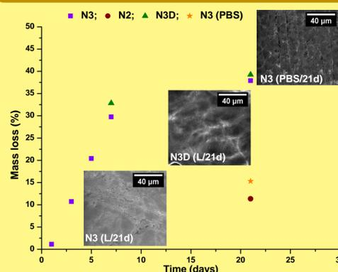
Figure 5. Graphical representation of the mass loss versus time of the formulations in the presence of lysozyme, and corresponding SEM images
