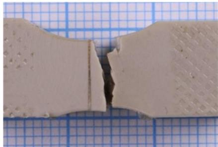
Fig. 6. The welded joints of the PEI and PEEK samples and their deconstruction at mechanical tests.
