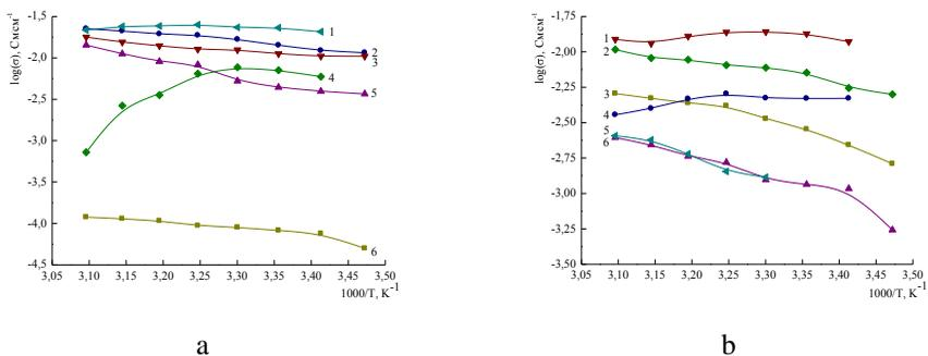
**Fig. 2.** Temperature (1000/T) dependence of ionic conductivity ( $\log\sigma$ ) ILPQSM: 1a–C-7-1, 2a–C-1-7, 3a–C-9-1, 4a–C-1-8, 5a–C-8-1, 6a–C-1-9; 1b–C-13-7, 2b–C-13-8, 3b–C-7-13, 4b–C-8-13, 5b–C-13-9, 6b–C-9-13
