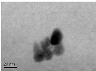
**Fig. 1.** TEM micrograph of PVP-stabilized nZnO sol.
