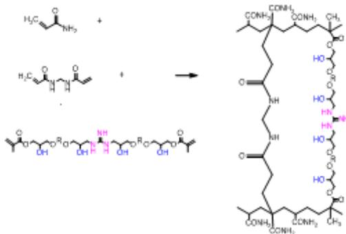
The scheme of synthesis of polyacrylamide hydrogel matrix, containing guanidine acrylic oligomer
