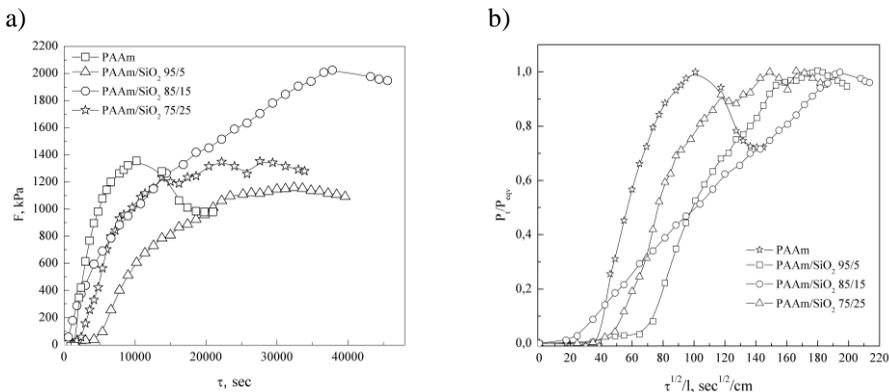
**Fig. 1.** Time-swelling pressure (a) and Fickian sorption curves (b) for PAAm/SiO<sub>2</sub> composites with SiO<sub>2</sub> content: 0, 5, 15 and 25 wt.%.
