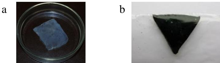
**Fig. 1.** Bacterial cellulose pellicle (a) and BC/PANI composite (b).
