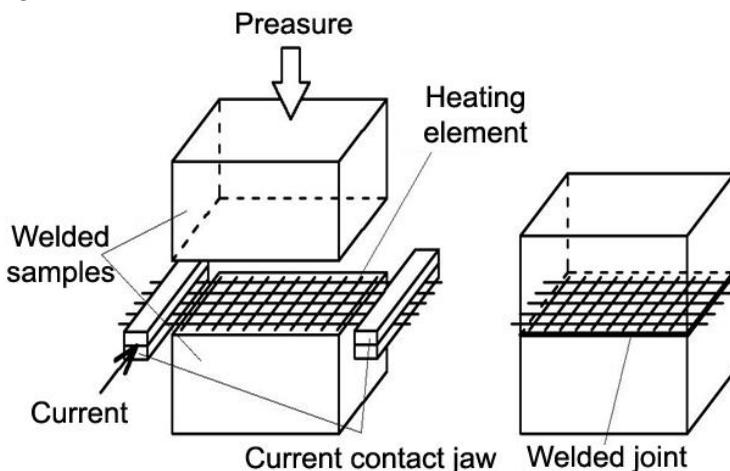
**Fig. 3.** The principal scheme of the thermistor welding.
