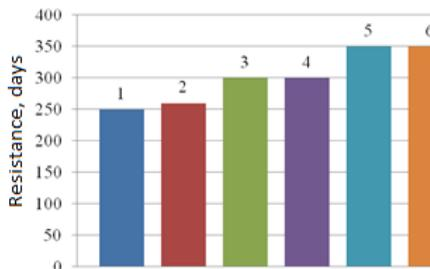
**Fig. 1.** Stable PU coatings in fresh water: 1 PUS; 2 PUS +Zn(60%); 3 PUS +Zn(60%) + NONO (1%); 4 PUP; 5 PUP + Zn(60%); 6 PUP+ Zn(60%) + NONO.
