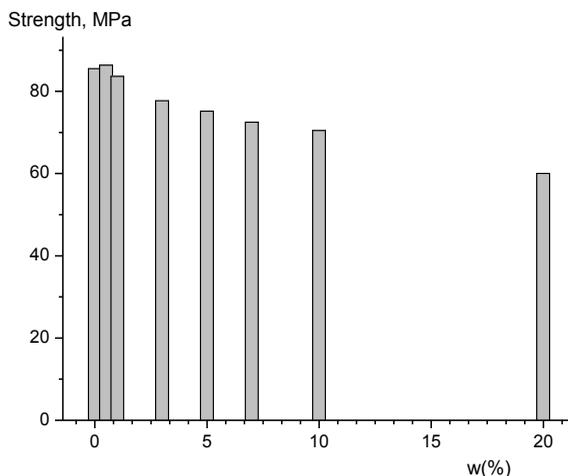
**Fig. 1.** Influence of the amount of Ep -Si on overall strength.
