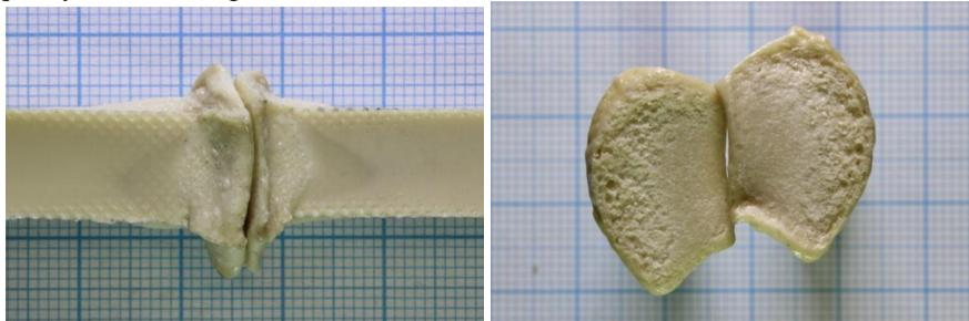
**Fig. 7.** The general view and character of the welded joint destruction of the PEI plates, obtained using butt welding with the heated tool.
