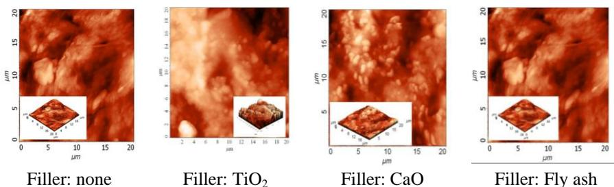
**Fig. 1** AFM Images of the all-wastes composites.
