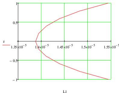
**Fig. 4.** Dependence between the layer thickness and strips position in the discs gap:  $w = 21 \text{ s}^{-1}$ ;  $h = 0.01 \text{ m}$ .
