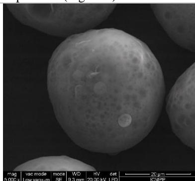
**Fig 1.** SEM pictures of VCL-MAC microparticles
