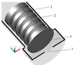
**Fig. 1.** Combined extruder: 1 – screw; 2 – body of extruder; 3 – disc; 4 – outlet.
