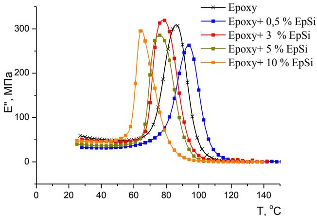
Fig. 3. Temperature dependence of the  $E''$  for epoxy.
