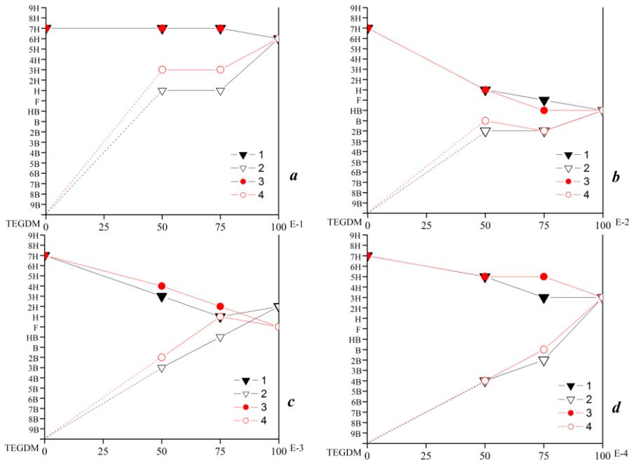
**Fig.** The dependence of surface hardness on the component ratio for IPNs on the base of E-1 (a), E-2 (b), E-3 (c) i E-4 (d), obtained by means of UV-lamp (1, 2) and sunlight (3, 4) in a closed and in an opened form, respectively.
