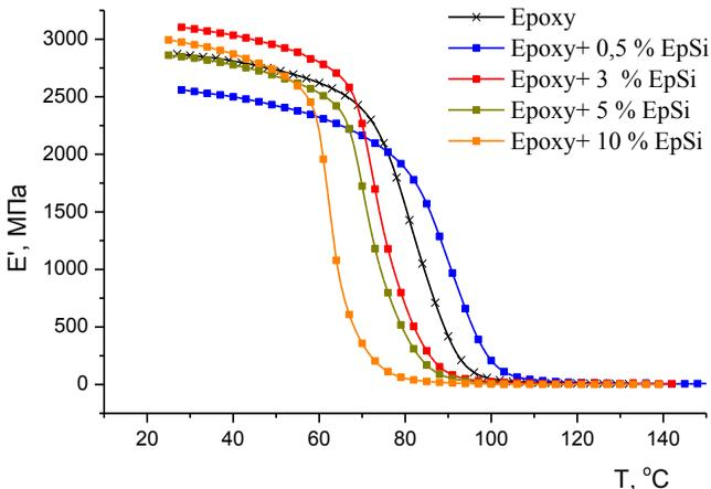
Fig. 2. Temperature dependence of the  $E'$  for epoxy.
