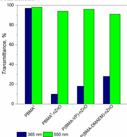
**Fig. 3.** UV-absorbance data of the polymers with immobilized nZnO at fixed wave length.
