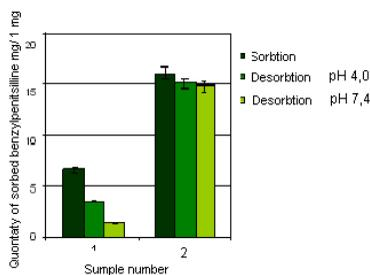
**Fig. 5.** Quantity of desorbed benzylpenitsilline polyacrylate matrix
