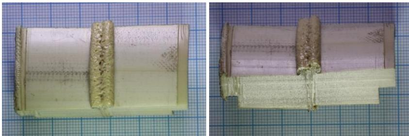
**Fig. 2.** The welded joint of the PEI pipes, obtained using the heated tool butt welding.
