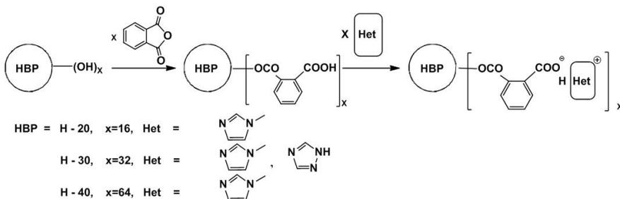
Synthesized OILs were characterized by FTIR and <sup>1</sup>H NMR spectroscopy. They are solid materials with low temperature of transition in viscous state in the temperature range 40-60°C. These compounds soluble in polar organic solvents. According to DSC glass transition temperatures of the OILs are about -15°C. The synthesized OILs is thermostable up to 150-180°C.
