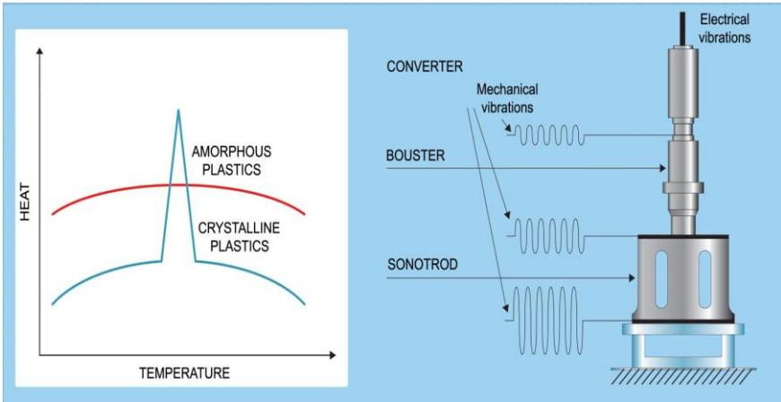
Fig. 5. The principal scheme of the ultrasonic welding.
