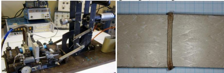
**Fig. 1.** The experimental equipment for butt fusion welding with the heated tool and the welded joint of the PEI plates, obtained using the heated tool butt welding.
