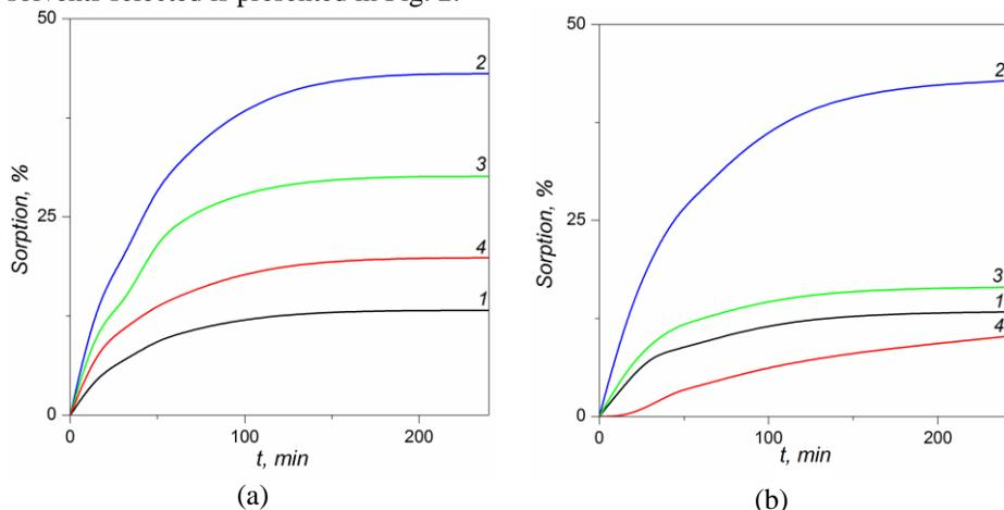
**Fig. 2.** Kinetics of sorption of EGME (a) and IPA (b) by polymer films: (1) PBMA<sup>5</sup>, (2) PBMA<sup>1</sup>, (3) P(BMA-VP), (4) P(BMA-DMAEM).
