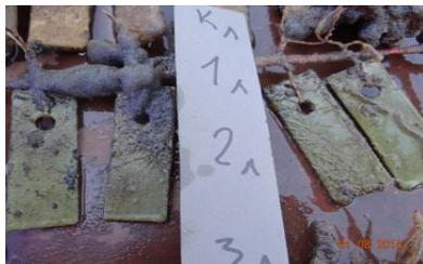
**Fig.4.** Fouling by zooperiphyton of control samples from vinyl plastic.
