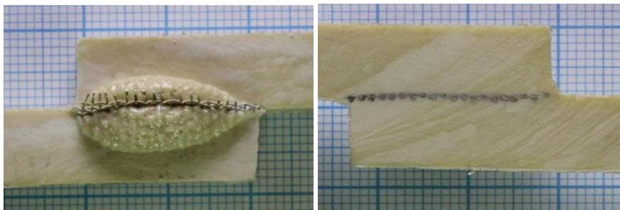
**Fig. 4.** The outward view and the cross-section of the lap thermistor weld of the PEI plates.
