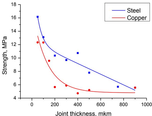
Figure 1. Influence of the joint thickness on overall strength for different substrates.
