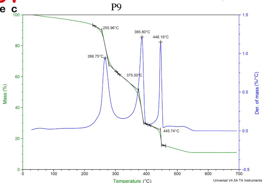
Figure 3. Thermogravimetric analysis and thermo differential analysis data of the thermal protection material with containing of microspheres 19% and density, 0,6 g/cm<sup>3</sup>.
