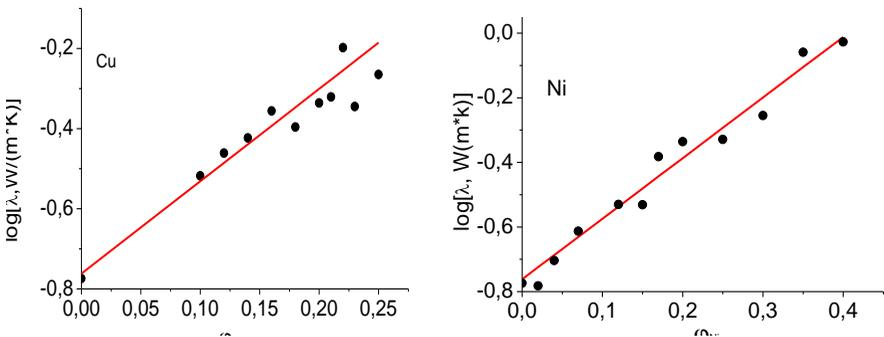
Figure 2. Experimental (points) and theoretical (solid line) concentration dependence of thermal conductivity on the content of Cu and Ni filler in epoxy matrix.
