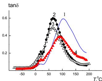
Figure 2. The temperature dependences of mechanical loss  $\tan\delta$  for OII-1 (1), OII-2 (2), OII-3 (3), and OII-4 (4).
