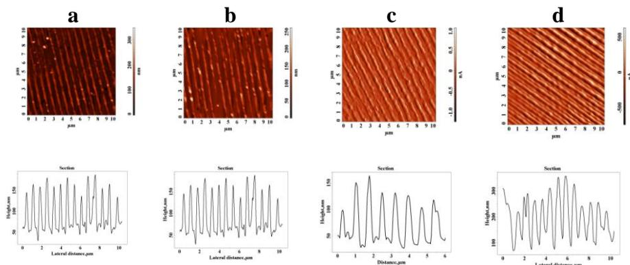
Figure 1. AFM images of the structured surfaces and diagram profiles of an azo-polyimide film after laser irradiation with  $10 \text{ mJ/cm}^2$  and  $45 \text{ mJ/cm}^2$ , by using 10 and 100 pulses.
