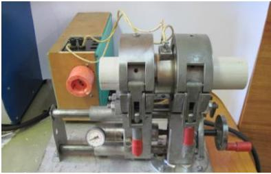
Figure 1. Multi-purpose device for traditional polymeric pipes hot tool butt welding equipped with the specific unit for welding within the limited volume.
