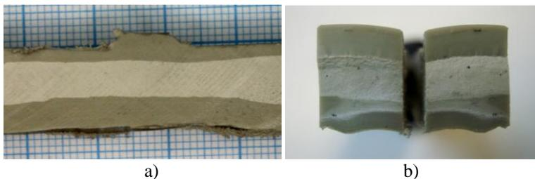
Figure 5. Cross-section of the specimen welded within restricted volume under optimal parameters before (a) and after (b) tensile test.
