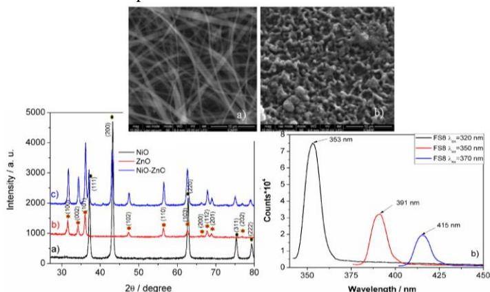
Figure 1. Properties of NiO, ZnO and NiO-ZnO/polysulfone composite nanofibers.
