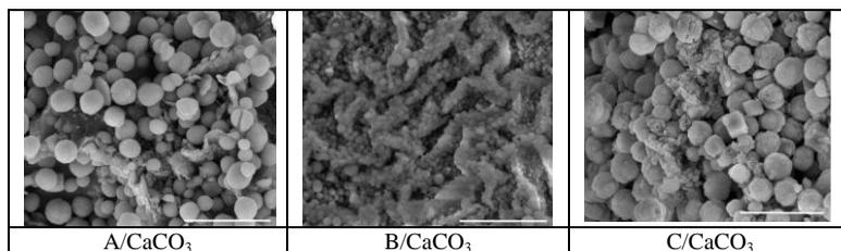
Figure 3. SEM images of beads surface after  $\text{CaCO}_3$  crystallization. Scale bar – 20  $\mu$ m.
