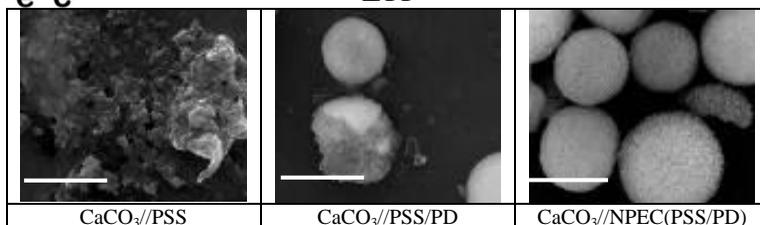
Figure 2. SEM images of some samples after EDTA treatment; PSS – poly(sodium styrene sulfonate), PD –poly(dimethyldiallylammonium chloride). Scale bar – 5  $\mu$ m.
