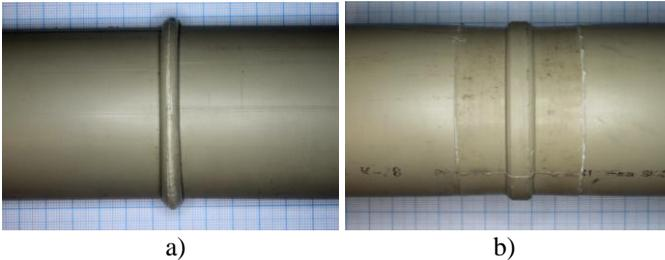
Figure 2. Welded joints of three-layer polypropylene pipes diameter 63 mm: butt welded (a) and welded within the limited volume (b).
