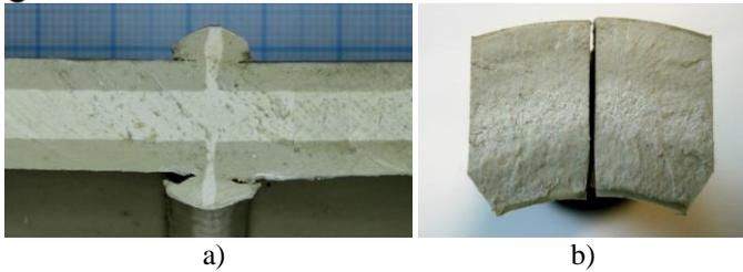
Figure 3. Cross sections of the hot tool butt weld (a), and general view of the destroyed specimen after tensile test (b).
