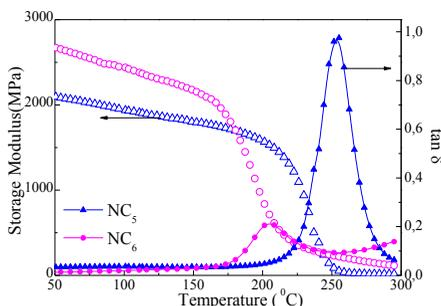
Figure 3. DMTA data for NC<sub>5</sub> and NC<sub>6</sub> samples.
