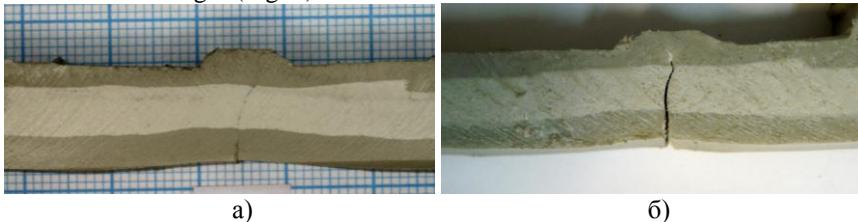
Figure 4. Cross-section of the specimen welded within the limited volume, with lack of fusion along the welding interface before (a) and after (b) tensile test.
