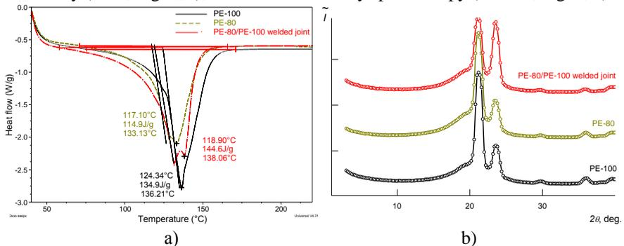
Figure 3. DSC (a) and WAXS (b) spectrums of pure PE-80, PE-100, and of their weld PE-80/PE-100.
