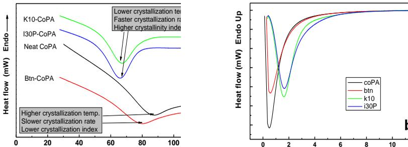
Figure. DSC analysis : a) Cooling scans and b) Isothermal crystallization.
