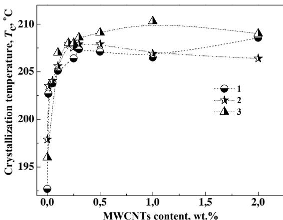
Figure 1. Effect of MWCNTs content and molding technique used on crystallization temperature  $T_c$  of the PBT crystallites in the PBT/MWCNTs nanocomposites studied: 1 – extrusion strand (series 1); 2 – hot pressing (series 2); 3 – injection molding (series 3).
