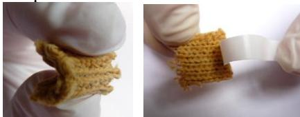
Figure 1. The obtained composite are flexible, robustly covered by polymer film (tape test).
