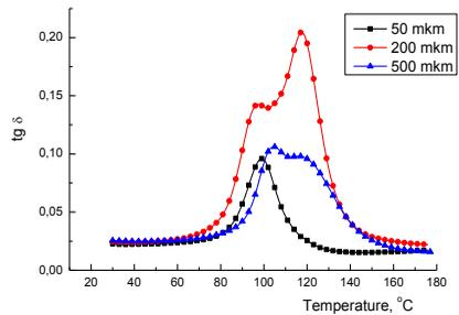
Figure 3. Temperature dependence of the  $\text{tg } \delta$  for copper adhesive joint.
