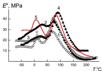
**Figure 4.** The temperature dependences of loss modulus  $E''$  for OII-5 (1), OII-6 (2), OII-7 (3), OII-8 (4), and IPN-2 (5).
