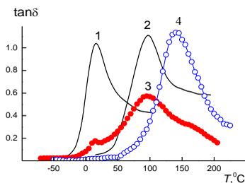
Figure 1. The temperature dependences of mechanical loss  $\tan\delta$  for PU (1), PHEMA (2), IPN-1 (3), and IPN-2 (4).
