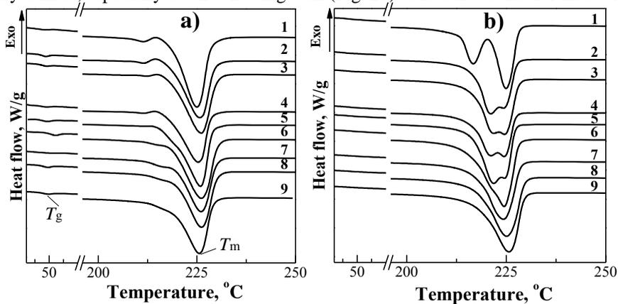
Figure 2. DSC thermograms for PBT/MWCNTs nanocomposites (extruded strands) with different content of MWCNTs, wt. %: 1 – 0; 2 – 0.01; 3 – 0.05; 4 – 0.1; 5 – 0.25; 6 – 0.3; 7 – 0.5; 8 – 1.0; 9 – 2.0; a) 1<sup>st</sup> heating scan; b) 2<sup>nd</sup> heating scan.
