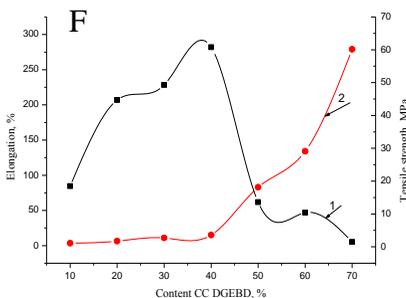
**F** - The dependence of mechanical properties of system (DER 331 + CC DGEBD) + DETA (schedule I):1 – tensile strength, 2 – elongation
