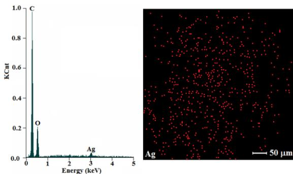
Figure 1. The EDX pattern, quantification data and corresponding EDX map collected from F1+2.5% Ag film.
