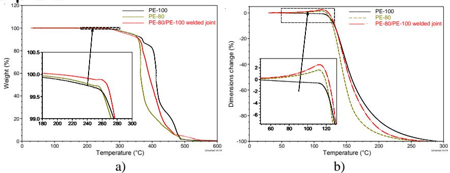
Figure 2. Thermogravimetric (a) and thermomechanical (b) results of pure PE-80, PE-100 and their PE-80/PE-100 weld.
