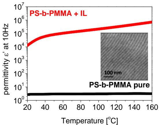
Figure 1. The permittivity value of pure PS-b-PMMA and of PS-b-PMMA doped with an ionic liquid. Insertion: sequence of insulating and conductive polymer nano-layers.
