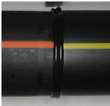
Figure. 1. Dissimilar pipes weld (PE80 and PE-100, 63 mm diameter).
