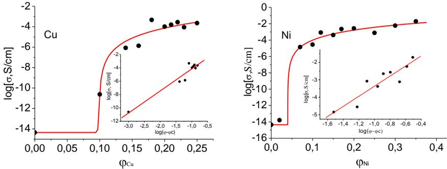
Figure 1. Experimental (points) and theoretical (solid line) percolation conductivity depending on the volume content of Cu and Ni filler in epoxy matrix.
