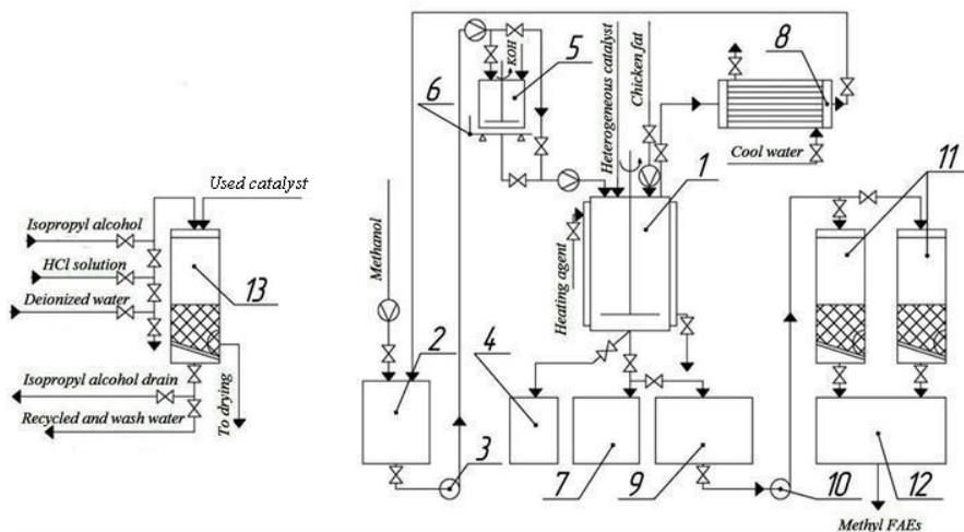
Figure 1. Process flow diagram for methyl FAEs production and catalyst regeneration unit:
