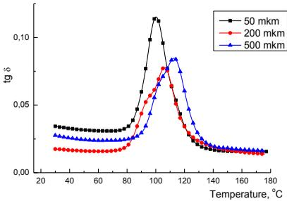
Figure 2. Temperature dependence of the  $\text{tg } \delta$  for steel adhesive joint.
