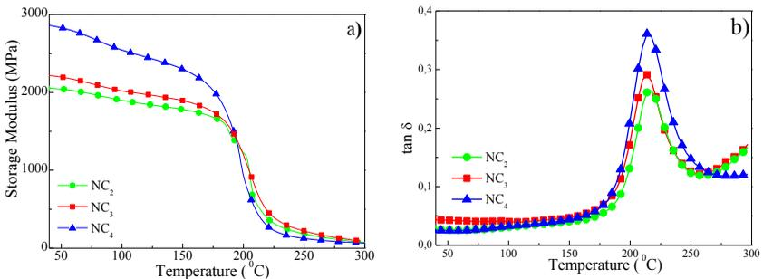
Figure 2. DMTA data for NC<sub>2</sub>, NC<sub>3</sub> and NC<sub>4</sub> samples.
