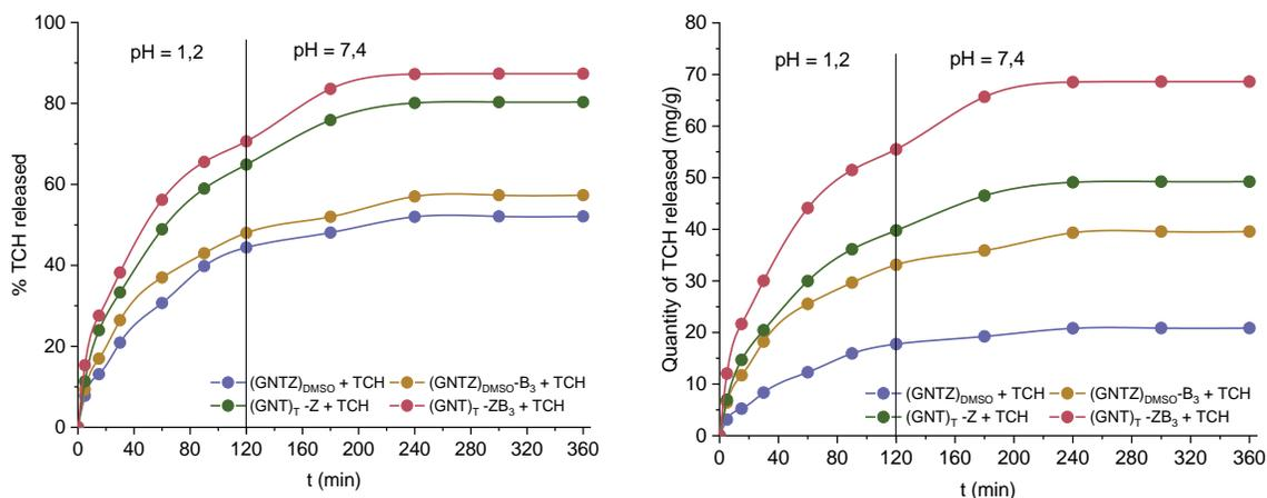
**Figure 6.24.** Release curves of TCH from  $(GNTZ)_{DMSO}+TCH$ ,  $(GNTZ)_{DMSO-B_3}+TCH$ ,  $(GNT)_T-Z+TCH$  and  $(GNT)_T-ZB_3+TCH$  microparticles.
