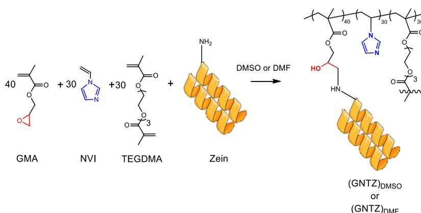
**Figure 5.2.** *Synthesis of hybrid zein microparticles by suspension polymerization.*
