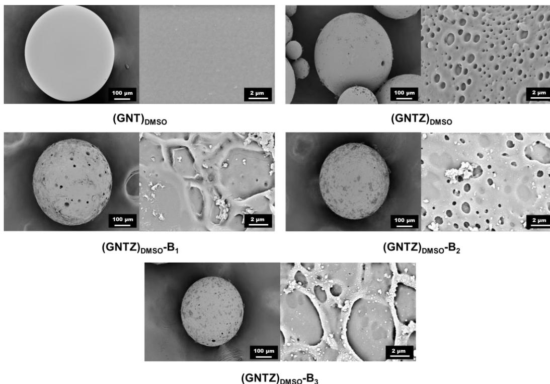
**Figure 5.13.** SEM images of zwitterionic hybrid microparticles synthesized by zein grafting during polymerization.
