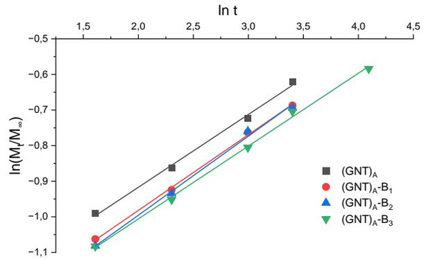
**Figure 4.11.** Plot of  $\ln(Mt/M_\infty)$  versus  $\ln t$  for (GNT)<sub>A</sub> microparticles before and after betainization.
