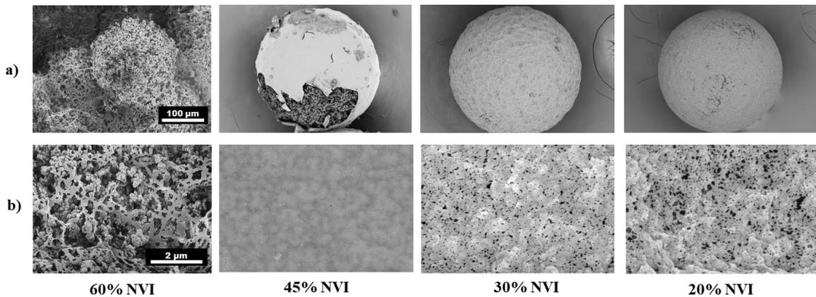
**Figure 3.3.** The influence of the molar percentage of NVI on the morphology of porous microparticles a) general look; b) surface appearance, in the case of using the EGDMA as crosslinker in a molar percentage of 10% (Trofin et al., 2023).
