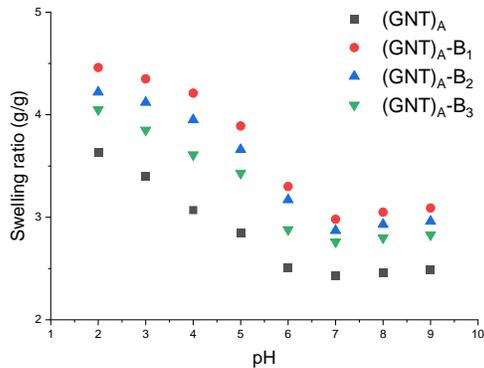
**Figure 4.8.** Swelling ratios at equilibrium of (GNT)<sub>A</sub> and zwitterionic microparticles in aqueous solutions with different pH values.
