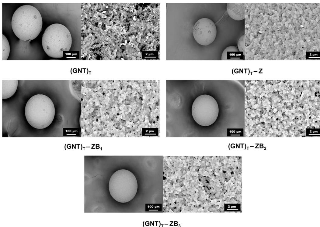
**Figure 5.14.** SEM images of the microparticles synthesized by post-polymerization grafting of zein, before and after grafting/betainization.
