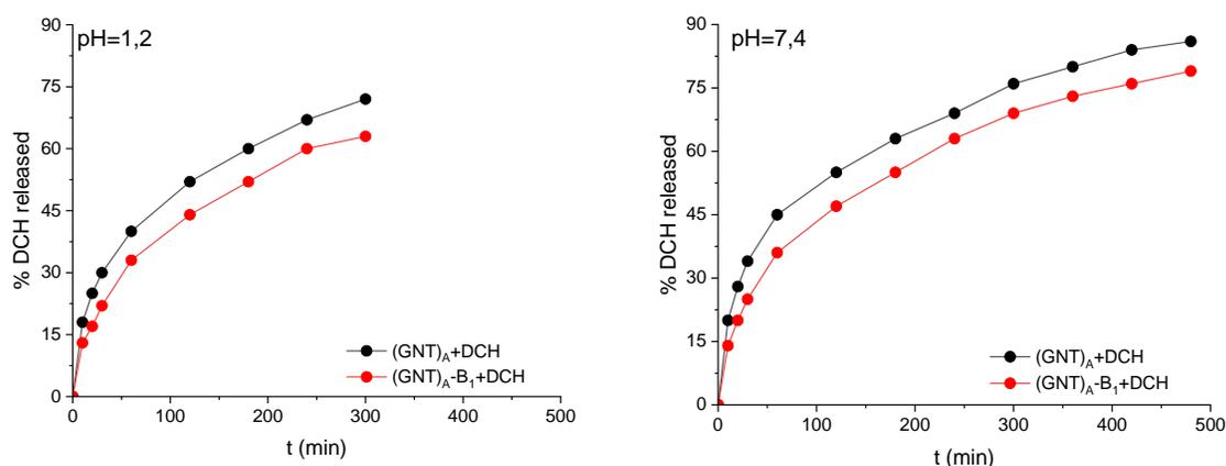
**Figure 6.12.** Release profile of DCH from  $(GNT)_A + DCH$  and  $(GNT)_{A-B_1} + DCH$  microparticles, at pH = 1,2 and pH = 7,4 expressed as a percentage.
