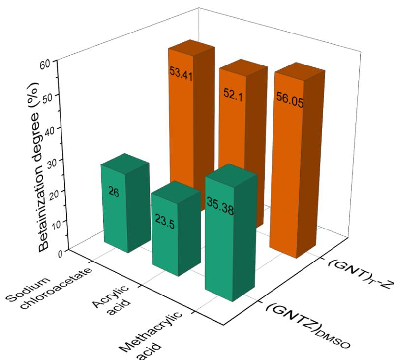
**Figure 5.11.** Betainization degrees of zwitterionic hybrid microparticles based on  $(\text{GNTZ})_{\text{DMSO}}$  and  $(\text{GNT})_{\text{T}}\text{-Z}$ .
