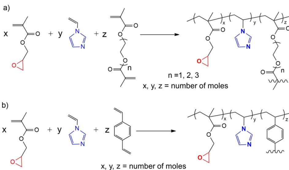
**Figure 3.1.** Copolymerization reaction between GMA and NVI using a) dimethacrylic crosslinker or b) divinyllic crosslinker (Trofin et al., 2022; Trofin et al., 2023).
