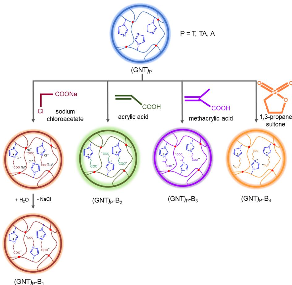
**Figure 4.1.** Schematic representation of the structure of porous microparticles before and after transformation with different betainizing agents.
