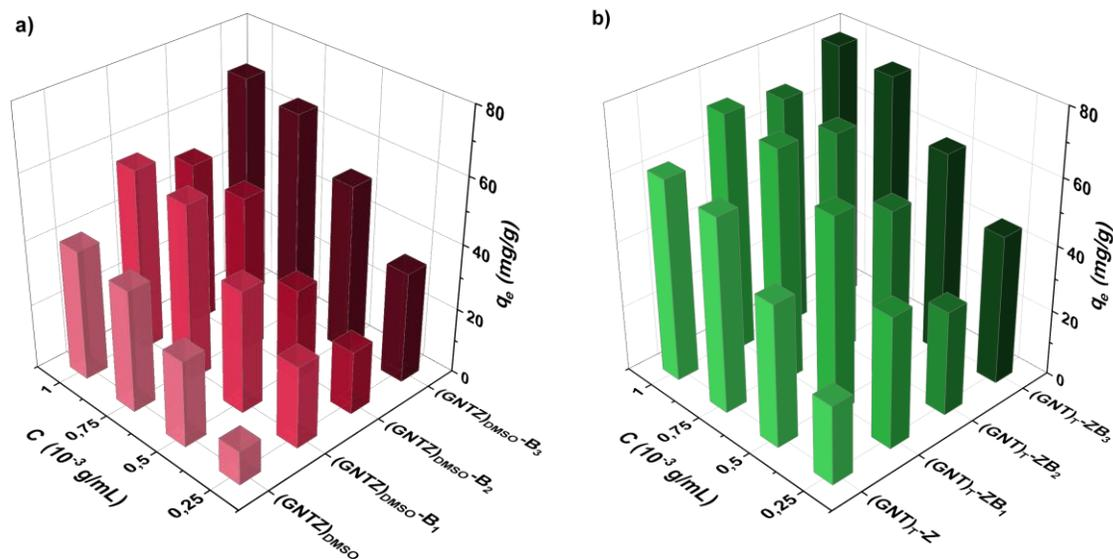
**Figure 6.21.** Amount of TCH sorbed by hybrid and zwitterionic hybrid microparticles obtained by zein grafting a) during suspension polymerization or b) after polymerization, for several initial TCH concentrations.
