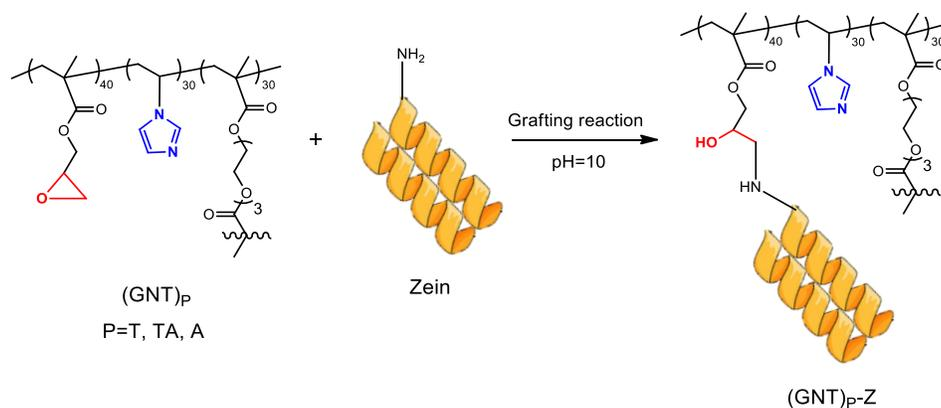
**Figure 5.4.** Zein grafting reaction on the surface of porous microparticles.
