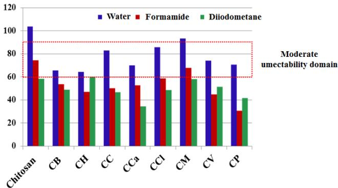
**Figure 18.** Mean values of the contact angle of the iminochitosan films with water, formamide and diiodomethane
