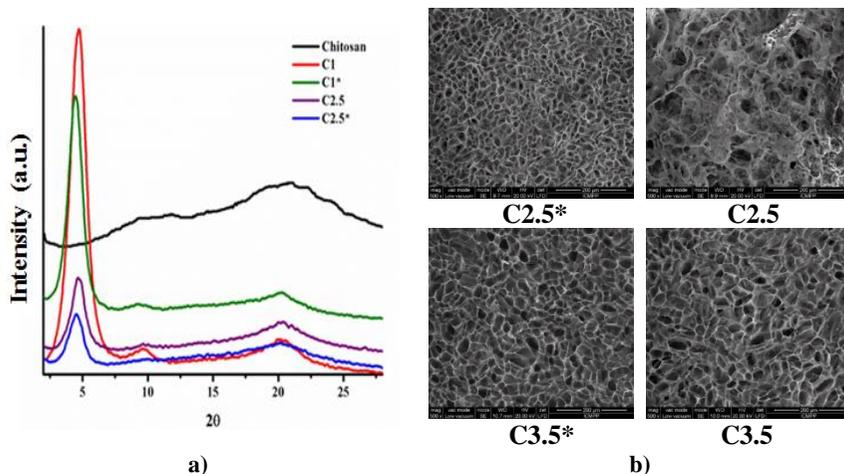
**Figure 38.** a )WXRd profiles and b) SEM microphotographs of representative hydrogels
