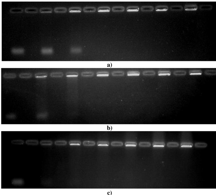
**Figure 51.** Agarose gel electrophoresis for a) ***JD1-bPEI800***, b) ***JD1-bPEI2000*** for  $N/P = 0.5; 1; 3; 5; 10; 20$  and c) ***JD1-PEG-bPEI800***, for  $N/P = 1; 3; 5; 10; 15; 20$ , at  $pH = 7.4$ ; naked DNA was used as control
