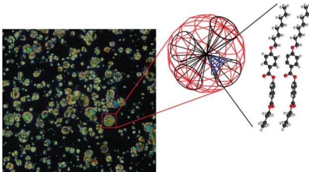
*Figure 95. POM image of a PDLC film and the topology of the Smectic A polygonal texture in a droplet*
