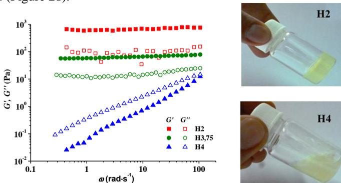
**Figure 28.** The dependence of  $G'$  and  $G''$  on the frequency for **H2\***, **H3.75\*** and **H4\*** at 37 °C and 1 Pa and pictures of representative hydrogels
