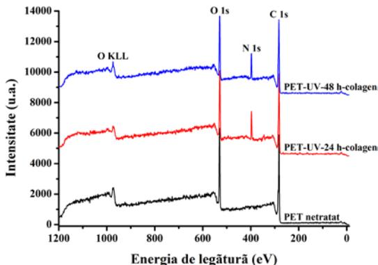
**Figure 8.** XPS analysis of untreated PET films and films with collagen immobilized on the surface.
